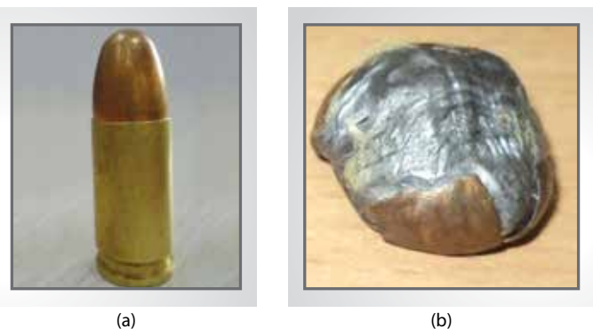
Figure 4: 9 \times 19 mm bullet (a) before test (b) stopped by fabric panel [3]
