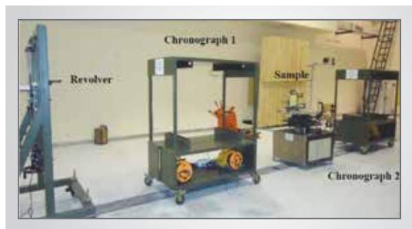
Figure 3: Ballistic evaluation of armour panel at TBRL, Chandigarh [3]
