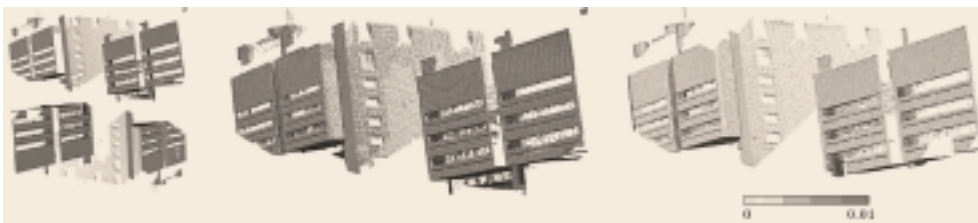
Figure 1: Given two building facades in arbitrary starting poses, we have designed algorithms that successfully align the scans. This is a challenging case for automatic registration since the scans comprise of noisy data with large flat featureless regions. This example has very few distinct features that can be reliably detected using any local descriptors.
